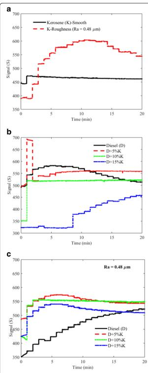
**Fig. 4** The dynamic signal (S) from different liquids recorded by the PS. **a** Kerosene (K), (**b**) authentic diesel oil (D) and the binary mixtures for the smooth surface. **c** authentic diesel oil and binary mixtures (D + K) for the rough glass with Ra =  $0.48 \mu m$
