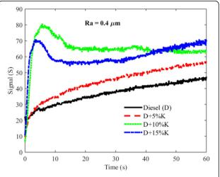
**Fig. 3** The dynamic signal (S) of the authentic diesel (D) and the binary mixtures (D + K) recorded by the TM sensor for the average roughness of Ra =  $0.4~\mu m$
