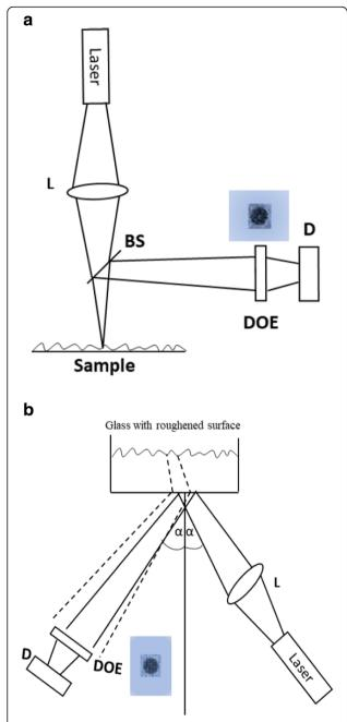
**Fig. 1** The schematics of the optical sensor (a) Table model (TM), (b) portable (PS). L is the focusing lens, BS is the beam splitter, D is the single-cell photodiode detector, and  $\alpha$ , the angle of incidence. The insert is the diffractive optical element (DOE) spatial filter
