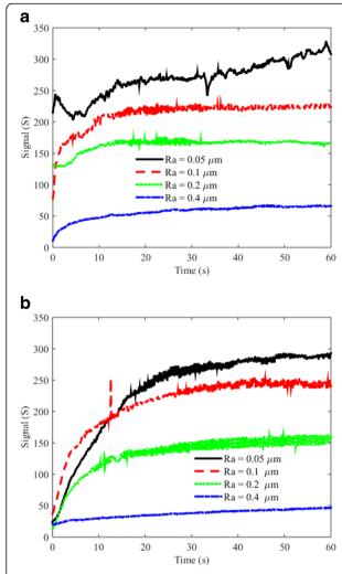
**Fig. 2** The dynamic signal (S) of the liquid samples recorded by the TM sensor. **a** Kerosene (K), (**b**) for the authentic diesel oil (D). Signal strength increases with time but decreases with the increase in metal surface roughness
