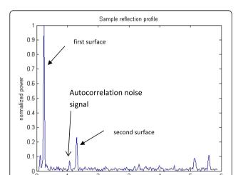
**Fig. 8** Layers positions of the glass sheet as measured using the ROCT method showing the autocorrelation noise signal highly reduced
