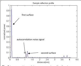
**Fig. 9** Layers positions of the same sample as Fig. 7a when measured using the OCT method showing the relatively high level of the autocorrelation noise signal
