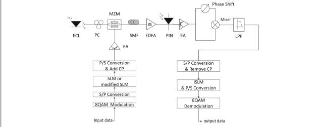
Fig. 2 8QAM-OFDM optical access system. ECL: external cavity laser. PC: polarization controller. MZM: Mach-Zehnder Modulator. EA: electrical amplifier. SMF: single mode fiber. EDFA: erbium doped fiber amplifier. PIN: positive intrinsic-negative. LPF: low pass filter
