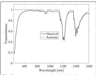
**Fig. 1** The transmittance curves of authentic diesel oil and kerosene samples. The hydrocarbons absorb NIR radiation in the vicinity of 1200 nm and 1400 nm
