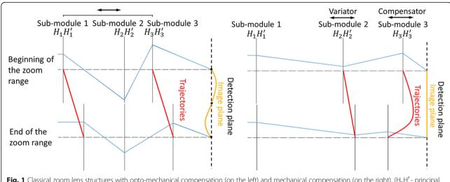
Fig. 1 Classical zoom lens structures with opto-mechanical compensation (on the left) and mechanical compensation (on the right),  $(H_xH_x'-principal plane of sub-module x)$
