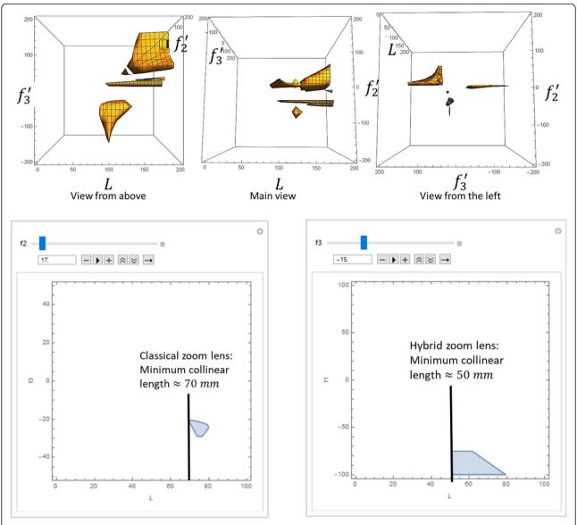
**Fig. 7** The collinear solution space for a classical zoom lens of the mechanical compensation type shown in Fig. 1 (above, requirements: V = 3,  $f'_A = 25$  mm,  $e'_{min} = 5$  mm,  $f'_{min} = 12,5$  mm) and the 2D analysis of the minimum collinear system lengths for the classical (lower left) and the proposed 'hybrid photographic zoom lens' (lower right)
