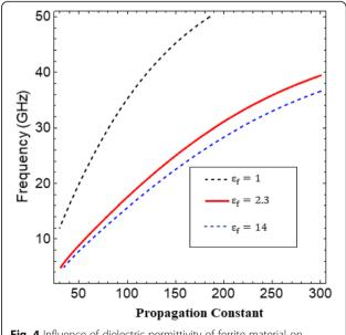
**Fig. 4** Influence of dielectric permittivity of ferrite material on propagation constant
