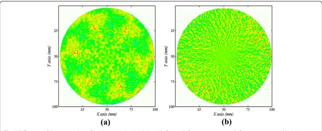
**Fig. 2** Differences of the averaged wavefront between *N* = 6 and *N* = 12 before and after compensation. **a** Before compensation, PV=8.27nm, RMS=0.80nm **b** After compensation, PV=6.30nm, RMS=0.70nm
