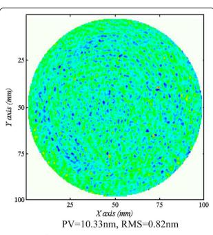
**Fig. 5** The difference of the averaged wavefront for N = 6 before and after position errors introduced
