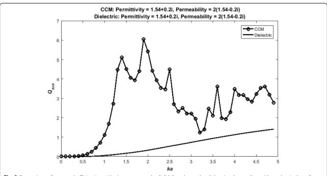
**Fig. 2** Comparison of scattered efficiencies with size parameter *ka*. Solid line shows the dielectric whereas line with marker is that of CCM sphere
