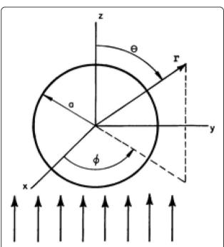
**Fig. 1** CCM Sphere having radius 'a' and spherical polar coordinate system  $(r, \theta \text{ and } \phi)$
