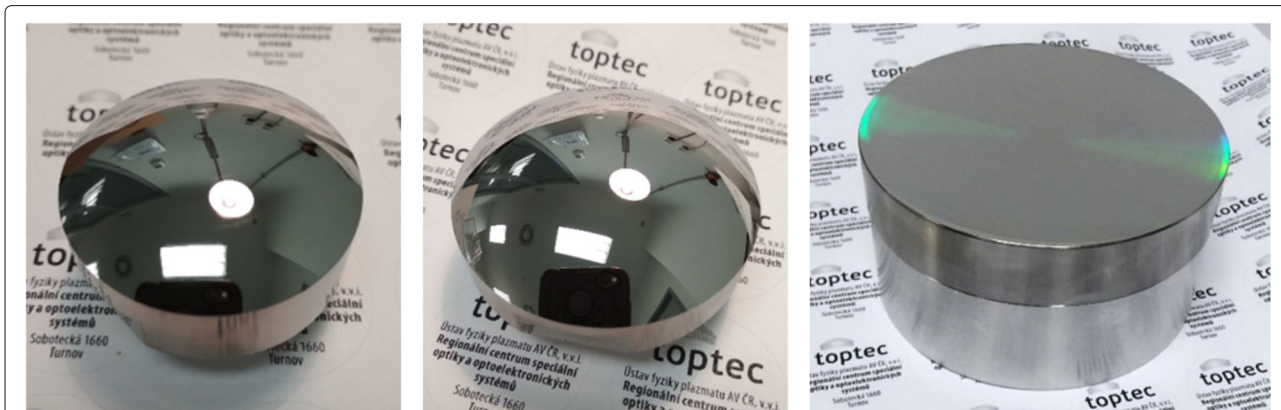
Fig. 1 Photos of the three specimens: The two-radii specimen (left), the convex toroidal surface (middle) and the concave toroidal surface (right)
