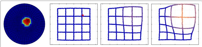
**Fig. 5** The temperature distribution on the lens after three seconds (left) and the images for t = 0s, t = 2s and t = 3s. The higher the changes in the refraction index due to temperature is, the more orange are the ray positions on the image plane. The red dot shows the center of the cylinder within which the heat is applied on the lens
