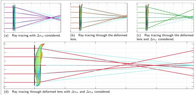
Fig. 4 Ray tracing through the single-lens system with different excitations considered. The blue dashed line always shows the ray tracing results for the ideal, unexcitated system
