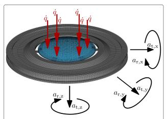
Fig. 2 Single lens optical system with thermal (red) and mechanical (black) excitation
