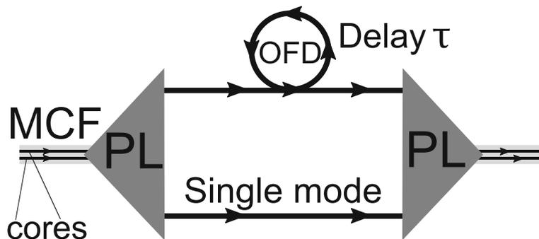
**Fig. 7** OFD device for codirectional modes. Light comes from the two cores of a MCF and is directed, via, for example, photonic lanterns, to a pair of parallel single-mode fibers. In one of them, an optic fiber delay is placed, introducing a delay  $\tau$  in one of the modes. Photons exit the SMFs through another PL and they are introduced back into the cores of an MCF
