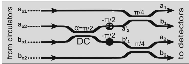
**Fig. 8** Bell-state measurement device for codirectional modes. A four port optical integrated circuit serves as a Bell-state measurement device for codirectional modes. Photons coming from Charlie's OC enter the device, where three DCs and two phase shifters implement the suitable operations. When light reaches the detectors the Bell states  $|\Psi^-\rangle$  and  $|\Phi^+\rangle$  are unambiguously identified, as required by MDI-QKD
