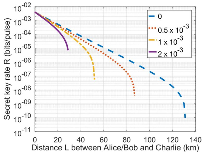
**Fig. 10** Secure key rate vs fiber length for different values of  $\alpha_{opt}$ . We set  $\alpha_{opt} = \{0, 0.5, 1, 2\} \cdot 10^{-3} \text{ km}^{-1}$ . Regarding the other parameters, the following values have been used:  $f = 1.16$ ,  $P_d = 3.01 \cdot 10^{-6}$ ,  $e_{opt} = 1.5\%$ ,  $\eta_d = 93\%$ ,  $\eta_c = 0.5$ ,  $\alpha_{att} = 0.2 \text{ dB/km}$ ,  $\mu_a = \mu_b = 0.36$  and  $\nu_a = \nu_b = 0.001$
