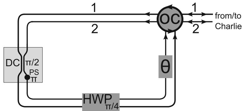
**Fig. 9** Autocompensating devices for codirectional modes and phase modulators. Light enters local loops through OCs. In the local loops, a DC with  $\kappa L = \pi/2$  plus a phase shifter introducing a phase  $\pi$ , for instance, in path 2. A HWP rotated  $\pi/4$  is placed for polarization autocompensation. Afterwards, a phase modulator is placed, so as to introduce the phase  $\theta$  and generate quantum states in order for Alice and Bob to encode their bits
