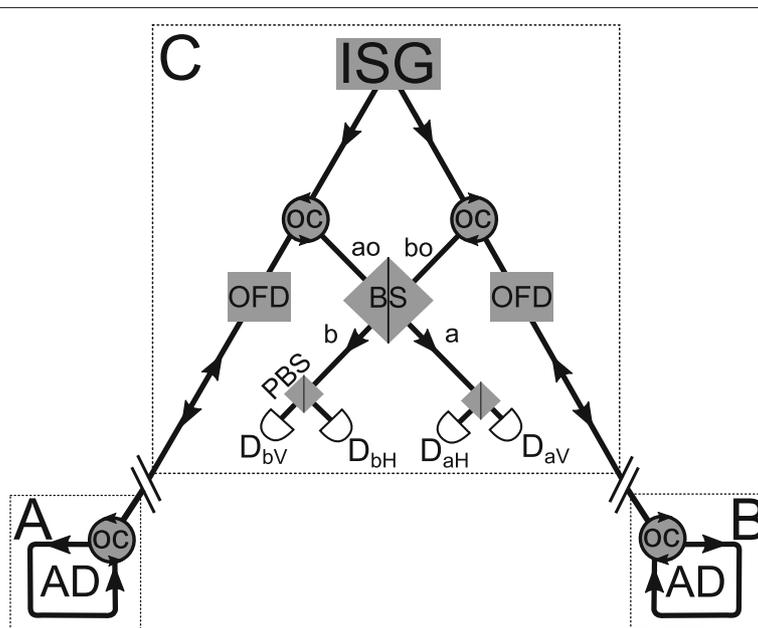
**Fig. 4** A-MDI-QKD system for polarization encoding. Charlie's generates suitable polarization states and launches them towards Alice and Bob. They autocompensate and modulate the relative phase between the horizontal and vertical components so as to encode their information. Light comes back to Charlie. Circulators redirect it to a polarization Bell-state analyser (Innsbruck scheme)
