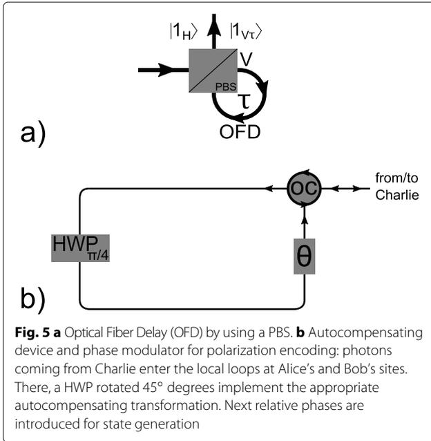
**Fig. 5 a** Optical Fiber Delay (OFD) by using a PBS. **b** Autocompensating device and phase modulator for polarization encoding: photons coming from Charlie enter the local loops at Alice's and Bob's sites. There, a HWP rotated 45° degrees implement the appropriate autocompensating transformation. Next relative phases are introduced for state generation
